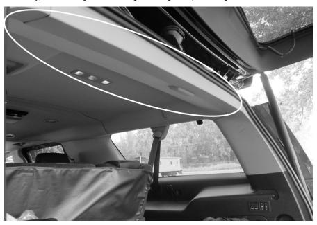
2. Alternately the light can be mounted to the trim above the window, on the rear hatch itself.
